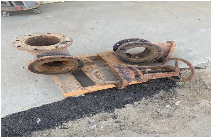
Old 8" Valve Removed dated 1940
